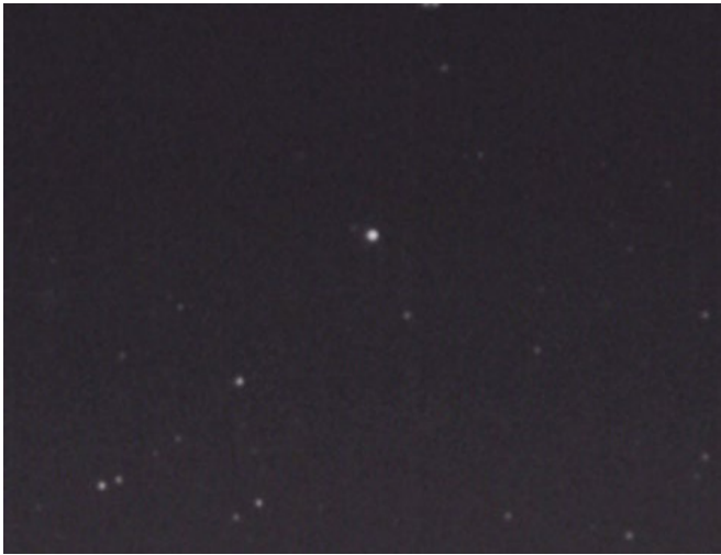
Figure 3: Partial frame from NTA movie of PBS buffer with 0.1% Tween ® , this view is typical of particle counts seen for the corresponding PSD.
